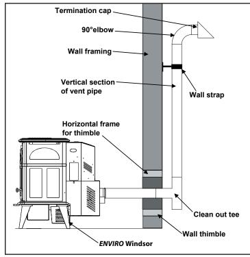
Figure 11: Through Wall with Horizontal Termination.
